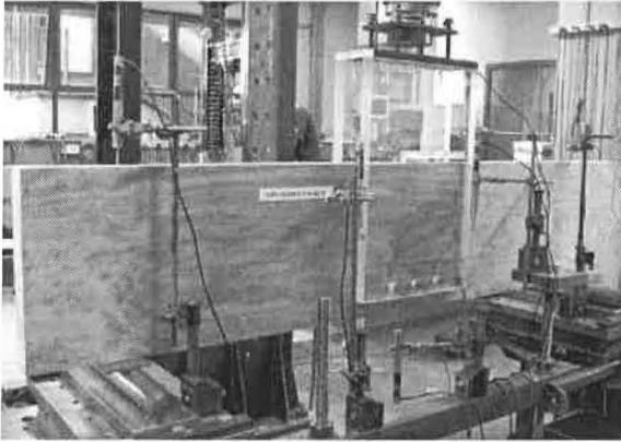
Figure 2: Test setup of LVL test series
