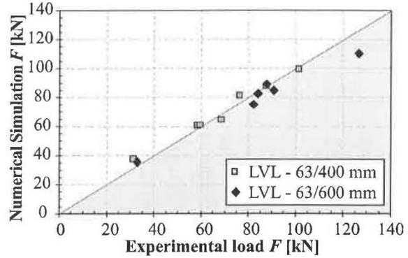
Figure 3: Correlation of the numerical model to test results in LVL
