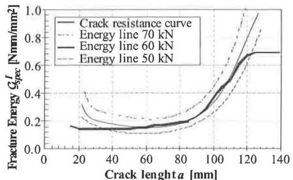
Figure 5: Crack resistance curve for mode I with energy lines for the outside side of the dowel marked in Figure 4
