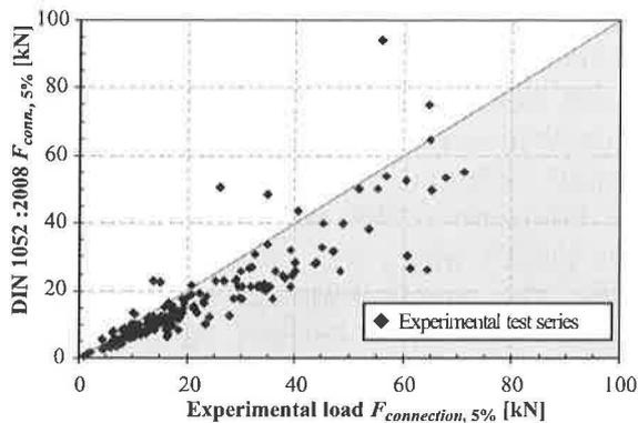
Figure 14: Comparison of DIN 1052:2008 and experimental test series published for European spruce or Canadian spruce
