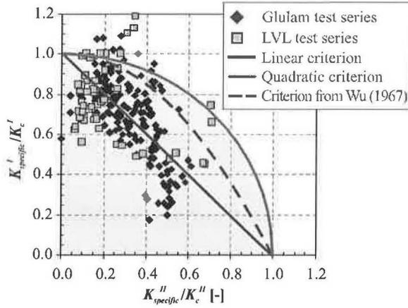
Figure 8: Failure criteria for dowel-type connections loaded perpendicular to grain for Glulam and LVL test series
