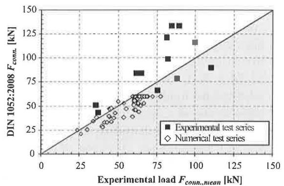
Figure 15: Comparison of DIN 1052:2008 and experimental as well as numerical test series for LVL
