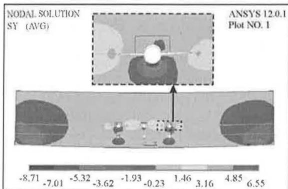
Figure 4: Numerical solution - transverse stress for 3 x 2 dowel type connection
