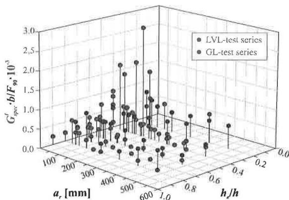
Figure 6: Distribution of fracture energies for mode I for Glulam and LVL
