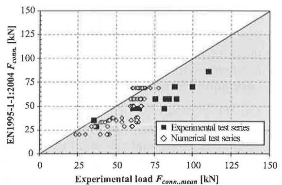
Figure 17: Comparison of EN 1995-1-1:2004 and experimental as well as numerical test series for LVL
