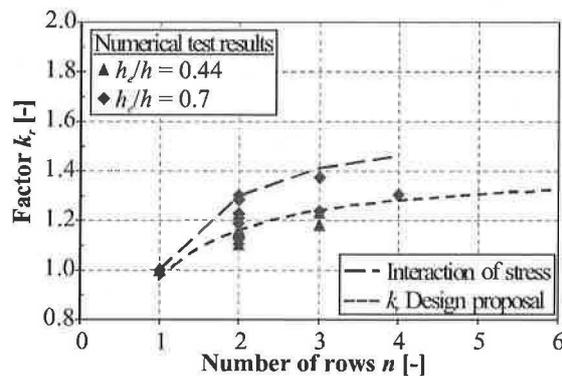
Figure 10: Factor  $k_r$ , depending on the numerical load capacities and stress situations determined
