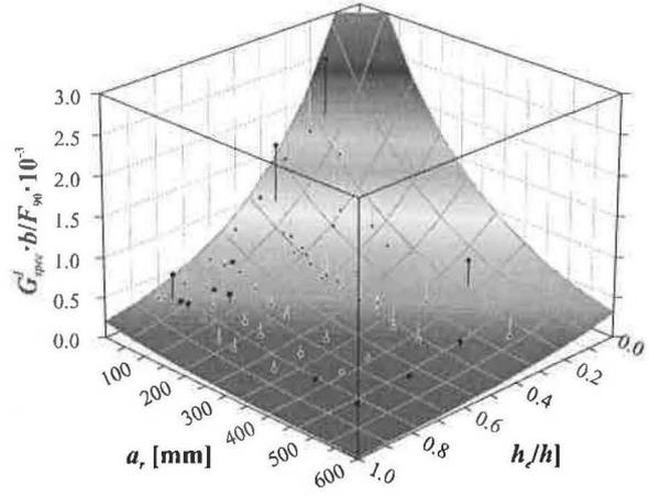
Figure 9: 3-dim. curve of the normalized fracture energies for mode I compared to the individual test results for solid wood/glulam
