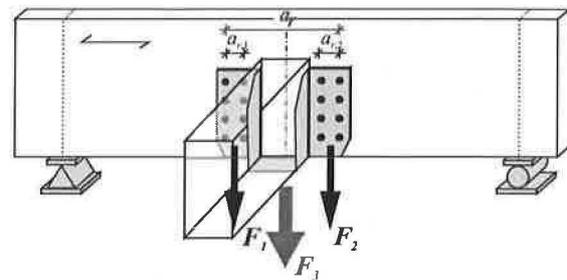
Figure 11: Design characteristics for nail plates or double dowel-type connections
