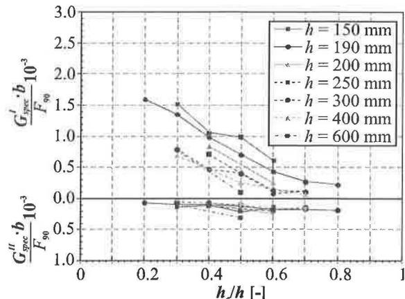
Figure 7: Dependency of fracture energies on depth of the member for Glulam
