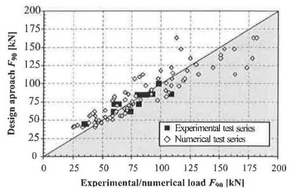
Figure 13: Comparison of design proposal and experimental as well as numerical test series for LVL
