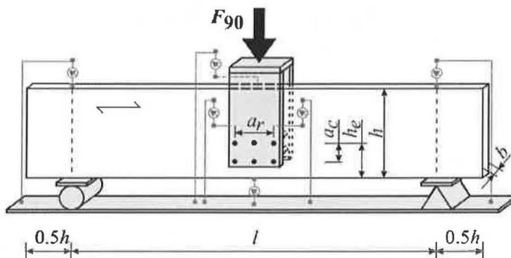
Figure 1: Test setup and connection layout defined
