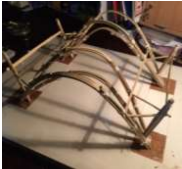
Figure 41: Fixing the supports and beams for using friction connections (Author)
