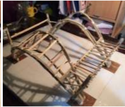
Figure 42: Adding the space truss supports using friction connections (Author)
