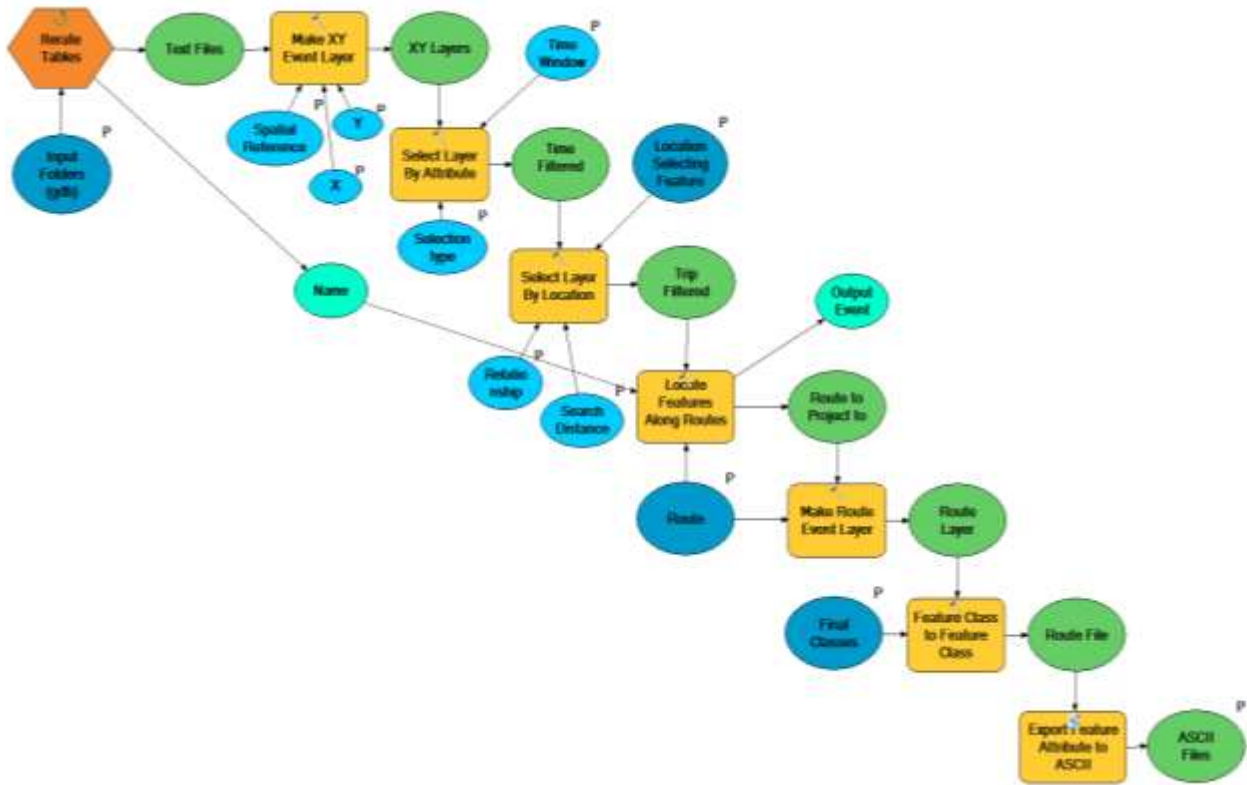
Figure 14: The GPS-LR tool workflow developed in ArcGIS ModelBuilder
