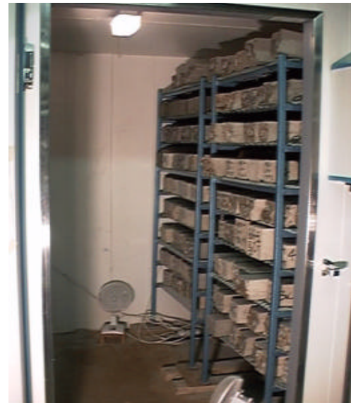
Figure 2. Retrofitted CO 2 system (Top): (a) monitoring/controller system, (b) injection system. The interior of the modified test carbonation chamber (Right)
