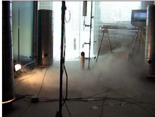
Figure 4 Concept evaluation by mockup tests (Displacement ventilation)
