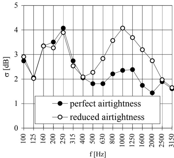
Figure 8. Standard deviation of the sound insulation test results for 156 windows with the same 4/16/4 glazing.
