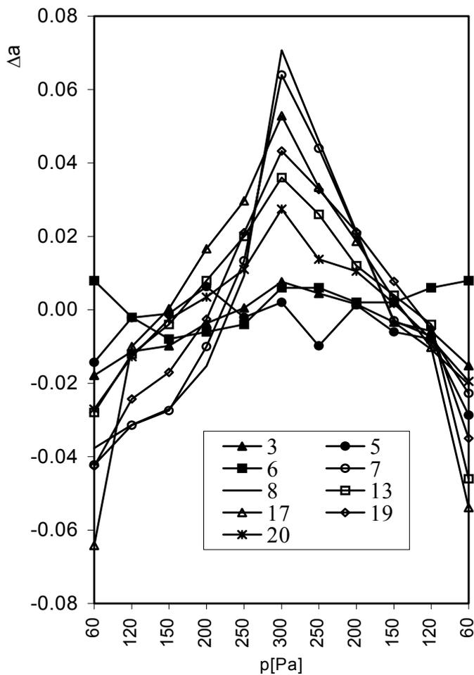
Figure 12. Averaged values of air permeability coefficient normalized to 0 for windows from analyzed systems No 3, 5, 7...
