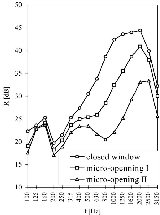
Figure 7. Sound insulation of single side hung casement window in different level of micro-opening.
