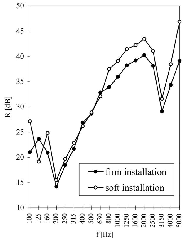
Figure 9. Influence of the method of a glazing installation in the frame on its sound insulation.
