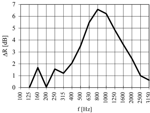
Figure 6. Decrease of sound insulation as an effect of window air tightness reduction, mean values.
