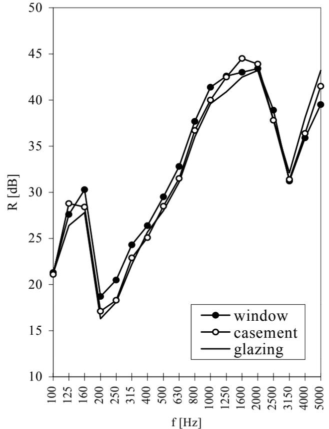
Figure 11. Measurement results; sound insulation of a single casement window, then the casement alone and the glazing removed from casement.
