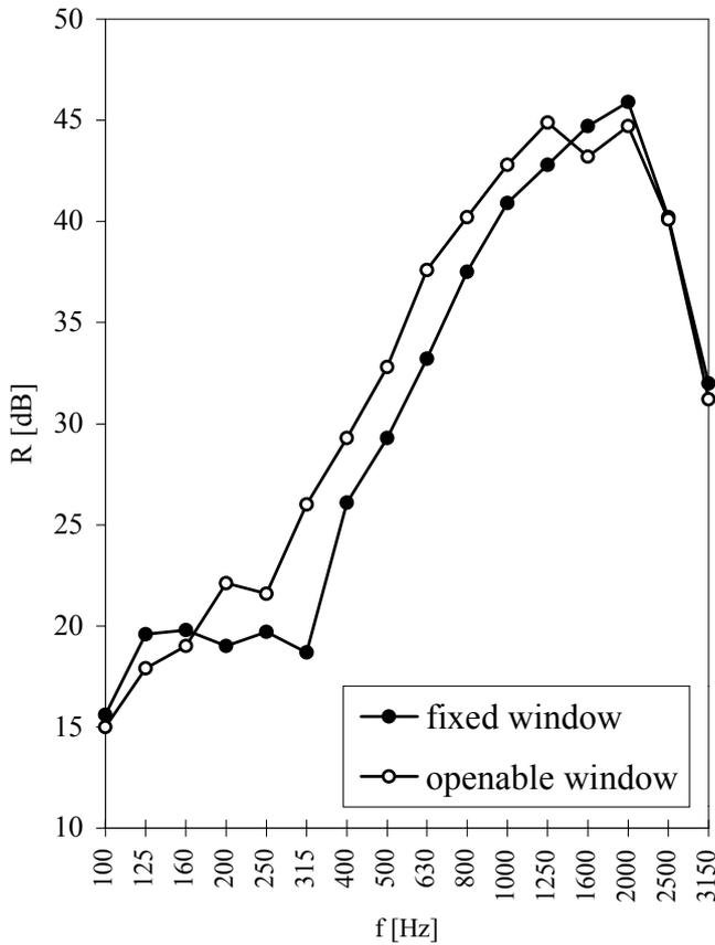
Figure 10. Measurement results; fixed and openable windows are taken from one manufacturer have the same dimensions and glazing.
