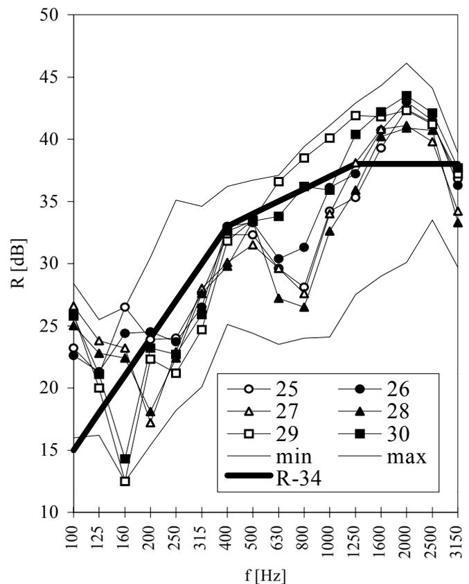
Figure 5. Windows from system No 5, reduced air-tightness.
