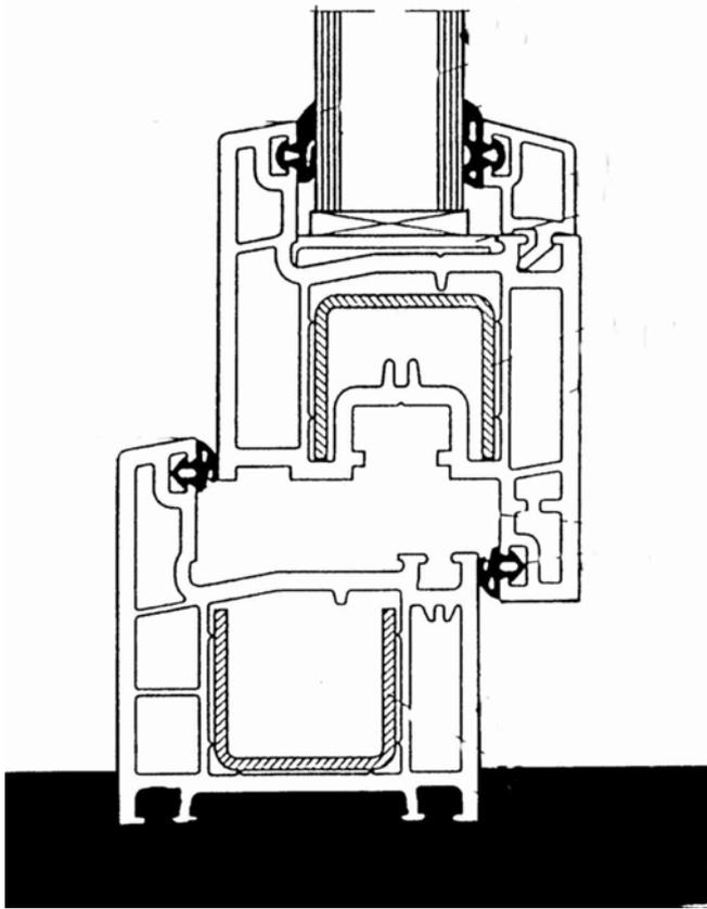
Figure 1. Cross section of window frame, joint between fixed and openable parts.
