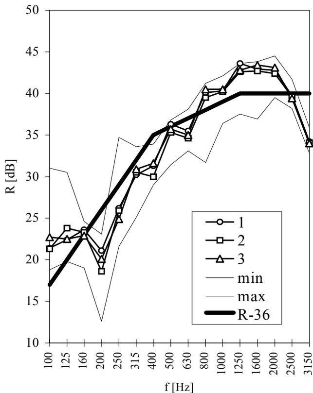
Figure 3. Sound insulation of windows with the same size and glazing, taken from one manufacturer.
