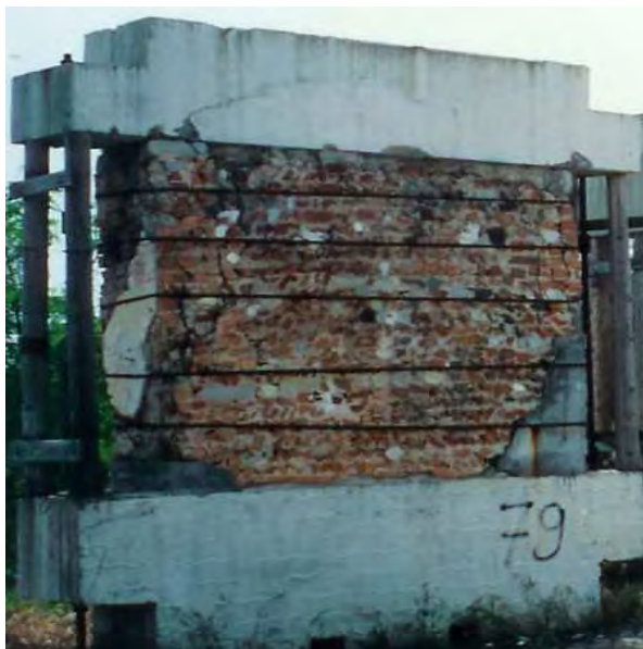
Figure 11: Specimen of masonry wall for a shear test in laboratory (21)
