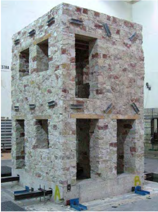
Figure 14: Shaking-table test of a masonry building at 2/3 scale (41)
