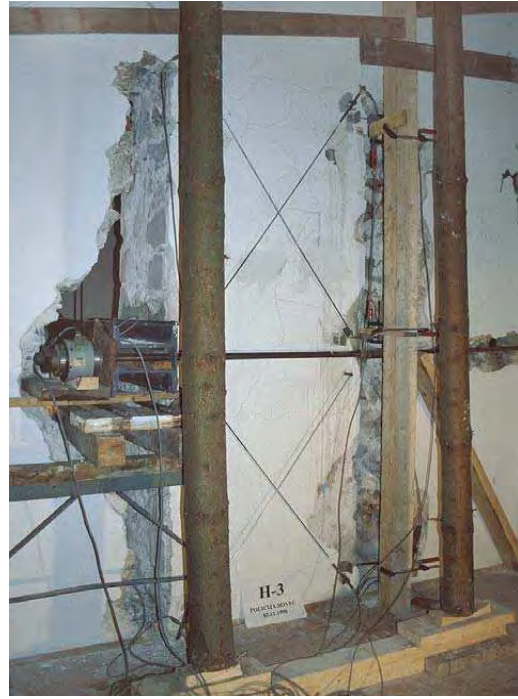
Figure 15: In-situ test of the lateral resistance of a masonry wall (26)
