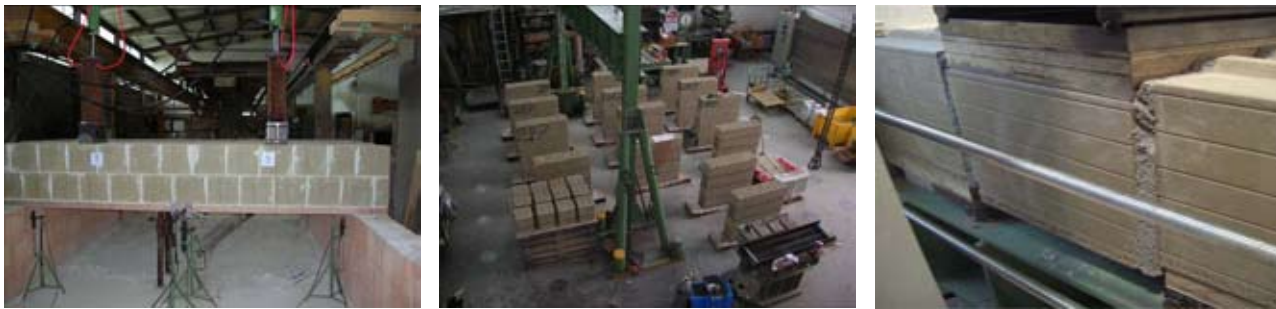
Figure 1: Several tests regarding the strength properties of the unfired loam brick walls have been done
