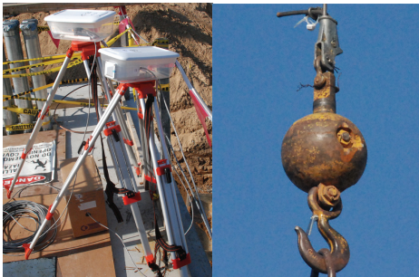
Figure 4 Sensor Field Setup, UWB Tag on Hook
