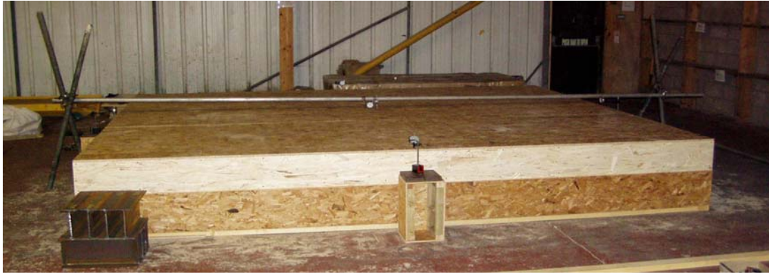
Figure 3: Setup for the deflection test
