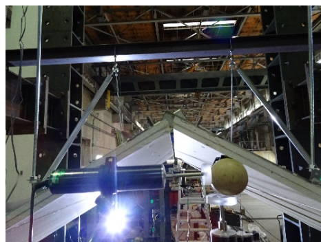
Photo 7: State of \delta = -5 mm. Gap occurs at slope-changing-part.
