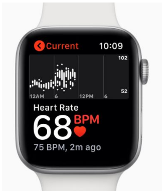
Figure 2a: Apple Watch Series 4 used for capturing heart rate of workers
