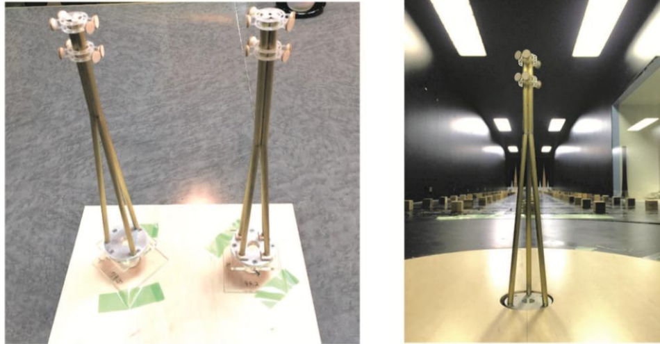
Figure 2: The experiment model used in the dynamic force balance test
