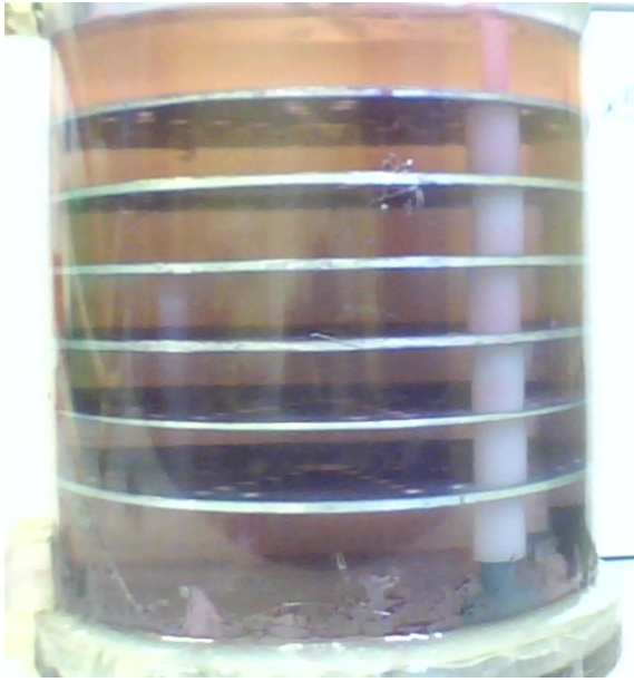
A) ECR1, Perforated electrodes.
