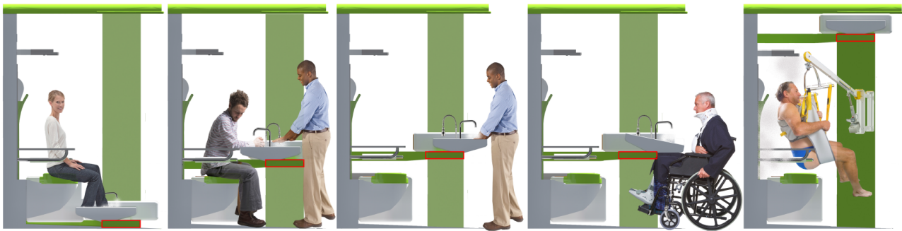
Fig. 5 The different possible positions of the sink and functionalities associated with them
