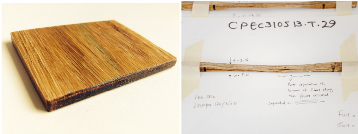
Figure 1. Left – High-tensile strength composite material as produced at the Future Cities Laboratory in Singapore. Right – Tensile test specimens after failure.
