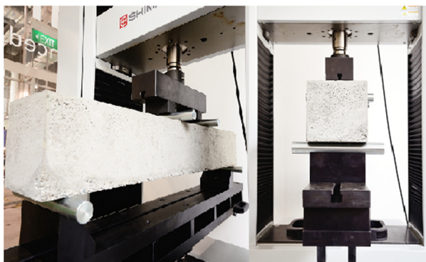
Figure 3. four point flexural strength test set-up
