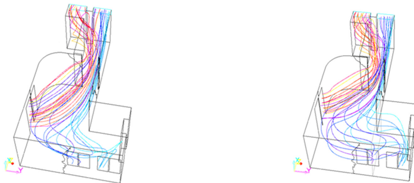
Figure 4. Flow lines for Area 1 generated with ANSYS Fluent. Cases 1 (left) and 4 (right).
