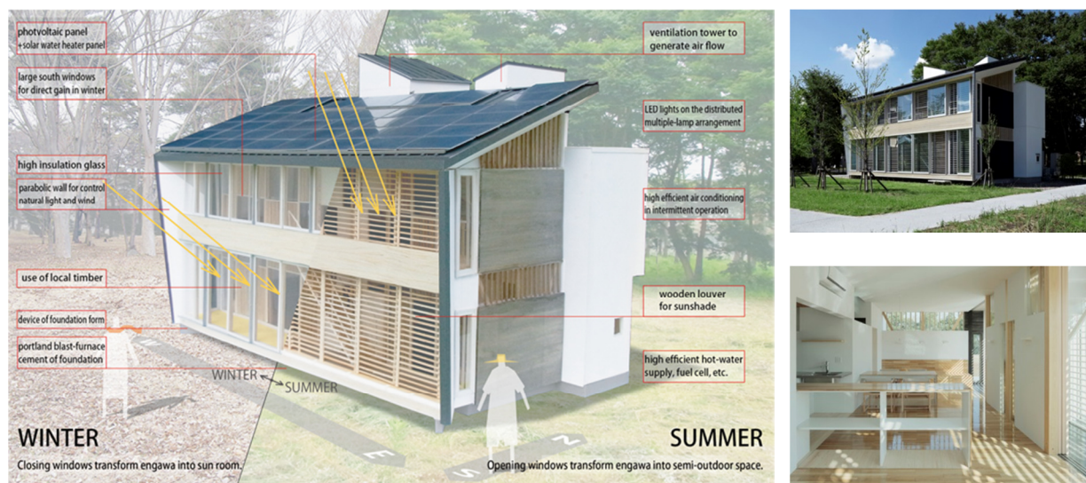
Fig.1 Design concept of the LCCM demonstration house (left) Photo.1* Exterior (right above), Photo.2* Interior of 1st floor * Photograph by Koichi TORIMURA
