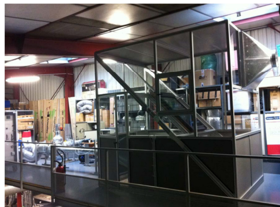
Figure 1: Test bench: aerodynamic chamber and regulated ventilator
