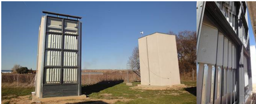
Figure 2. Experimental set-up located in Puigverd de Lleida (Spain). Left: ventilated facade and double height reference. Right: macro-encapsulated PCM inside the air cavity.
