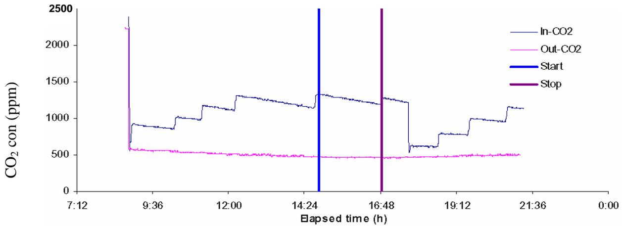
Figure 2a Decay curves of CO<sub>2</sub> under AER=0.1 conditions in chamber
