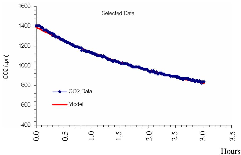
Figure 3b Simulation for selected data, AER<sub>simulation</sub>=0.34.
