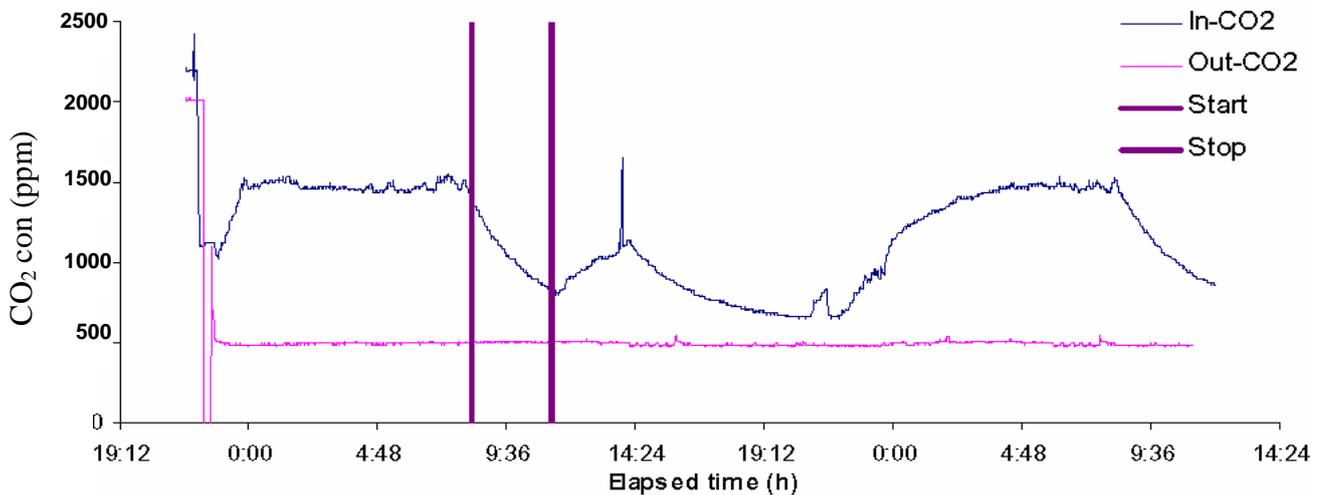
Figure 3a Decay curves of CO<sub>2</sub> in a apartment.
