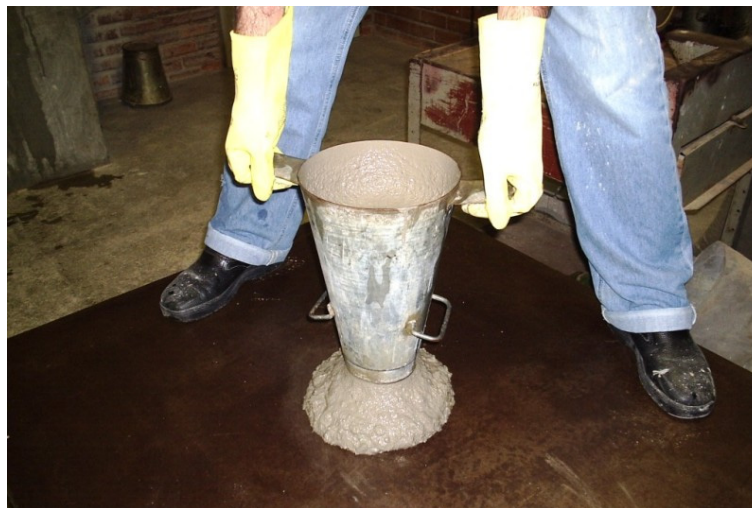
Figure 4 Inverted slump flow test
