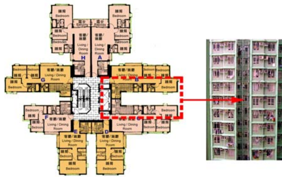
Figure 1 the red rectangular shape represents to an open area prescribed by local building regulations to permit the permeability of daylight and natural ventilation to habitable rooms such as kitchen, bathrooms and bedrooms. Described as a Re-entrant, such spatial arrangement is found to be a potential environment contaminant for the spread of bacteria due to poor ventilation and build-up of heat due to air conditioners.
