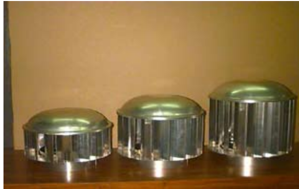
Figure No. 3. Variable blade height / Long Volume Turbines (LVT's)
